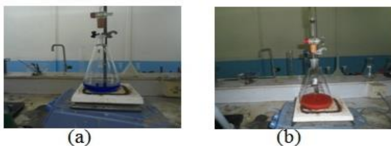
Figure 1: Experimental observation of Fehling method for total sugar determination (a) before titration, (b) at end point (brick red color), and formation of red precipitate due to \text{Cu}^{+1} formation
